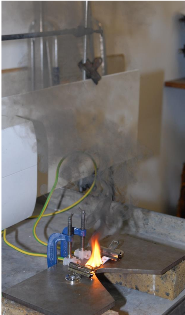
Note the strong flame and large amount of toxic smoke being produced from the small plastic sample.
